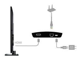
There will be an HDMI cable and USB adapter inside of the box, use the 5V-1A DC adapter to power up EZCast LAN box, and plug HDMI cable into HDMI port. We also suggest connect RJ045 port with your router to simplify setup procedures and get stable connection.
