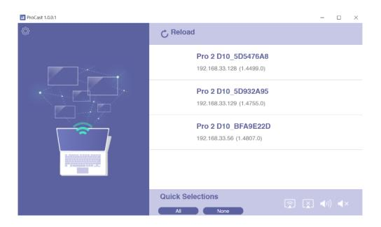
iii. Select the dongles that connected to output screens. By clickingat the bottom right of the page, you may start casting.
